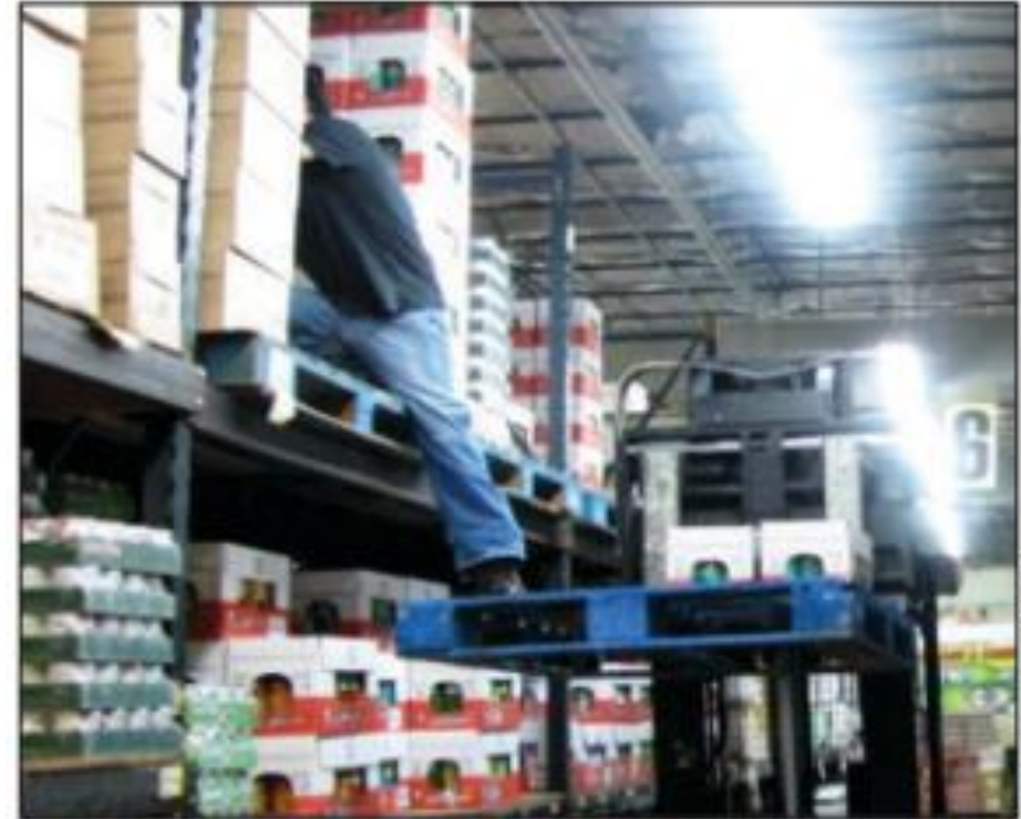
Figure 1: Example of a worker unsafely pulling inventory on a raised pallet.
